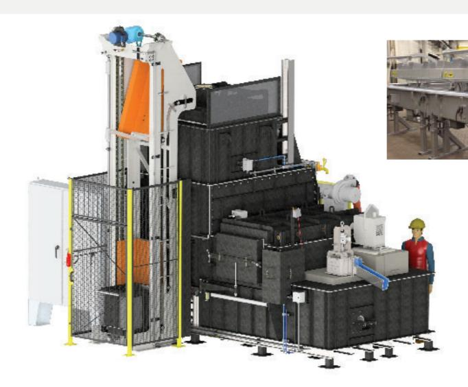
The Tower Melter was designed to allow for many different ways to move metal from the melter to the casting line. This includes HPDC, LPDC, Sand Casting, and any other form of casting that requires molten aluminium.
