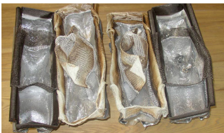
Distributor deformation and retained oxides—TF combo bag vs. standard combo bag.
