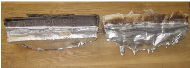
Distributor deformation and retained oxides—TF combo bag vs. standard combo bag.
