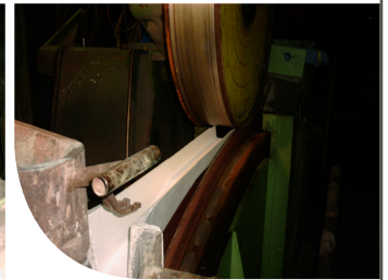
RFM Casting Spout just clears the Continuous Steel Belt
