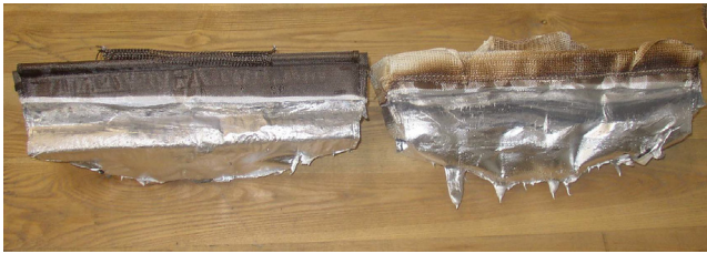
Distributor deformation and retained oxides—TF combo bag vs. standard combo bag.
