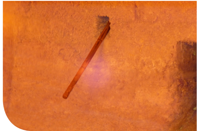
Pyrotek cast iron thermocouple protection tube in a furnace.
