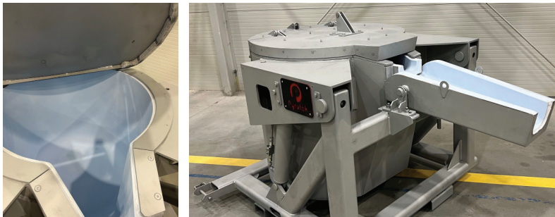
Precast refractory liner has excellent material properties due to casting, curing and firing processes.
