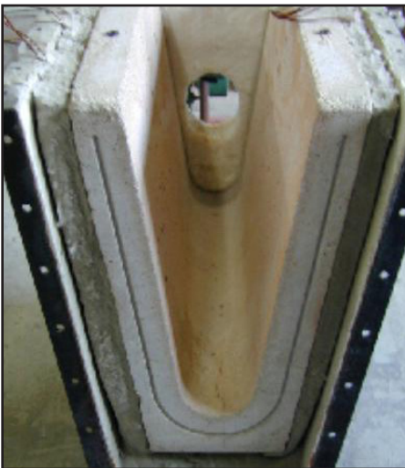
Pyroflow (L&D) Sintered Layer
