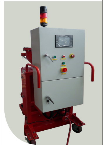
FIM-S5 with PLC Touch Screen Control
