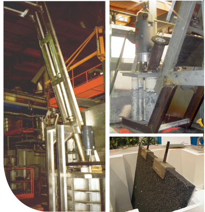
Left, Pyrotek M-30 transfer pump with piping. Top right, M-30 pump and impeller. Bottom right, Pyrotek BPF vertical gate filter.
