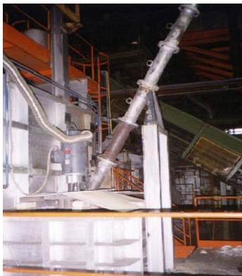
Pyrotek designed an M-30 pump with piping to lift metal from the basement to the first floor of the foundry.
